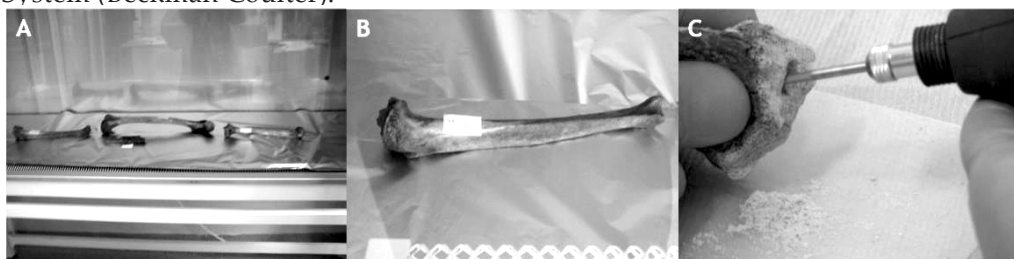
Fig. 2: Samples preparation steps: (A) drying after sodium hypochlorite wash, (B) UV exposure, and (C) bone powder sampling
